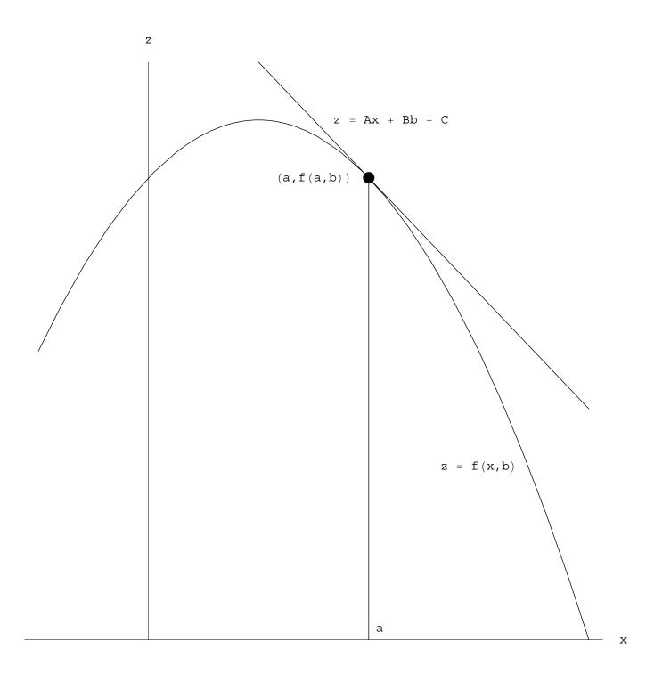
The section is a graph with a tangent line. We already know how to handle this. For clarity write g(x) = f(x, b): so that:
